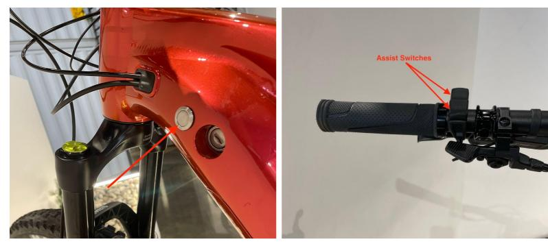
You can also hold down the lower assist button to engage walk mode. "Walk" will show on the display, and the drive unit will propel the bike forward as you walk with it. Push the upper button to return to the previous assist mode, or the system will automatically change back after one minute of inactivity.
