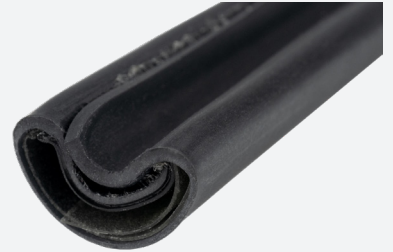
Photo 3: Overlap seams curled up prior to full shrinkage.
