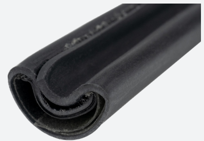
Photo 6: Overlap seams curled up prior to full shrinkage.
