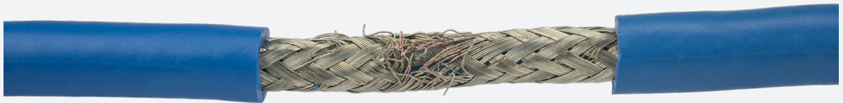
Photo 4: Insulation removed around braid damage
