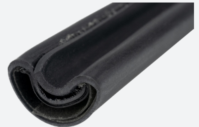
Photo 10: Overlap seam curled up prior to full shrinkage.
