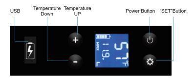
• Power On/Off: Press the Power Button (1) to turn the unit on/off
