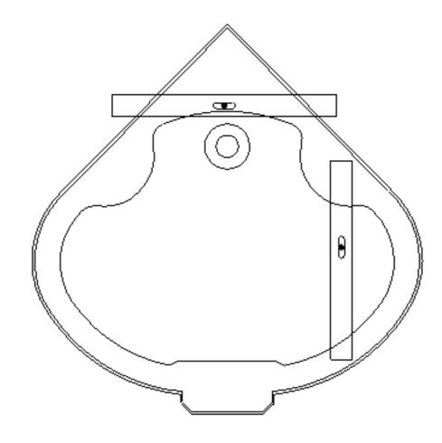
2. Adjust the shower tray to make sure the upper surface of the track is vertical with the wall. The upper side of the shower tray shall be level and all the legs shall reach the floor.
