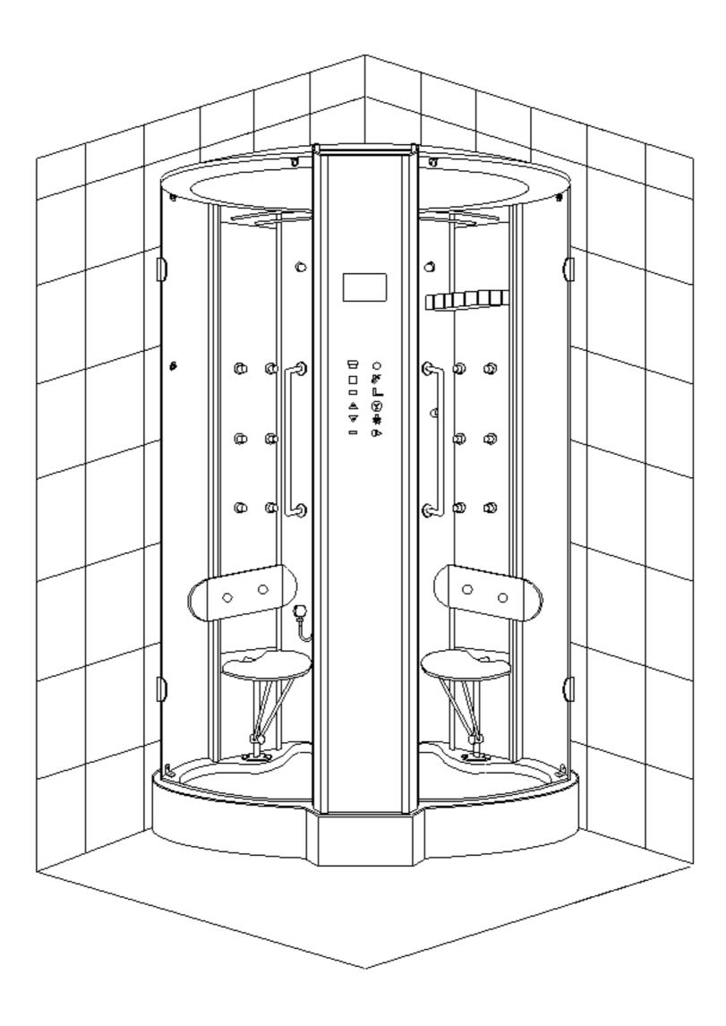
25. Get water supply and power supply connected and push the steam room against wall. No use within 24 hours until the silicone is completely dry.
