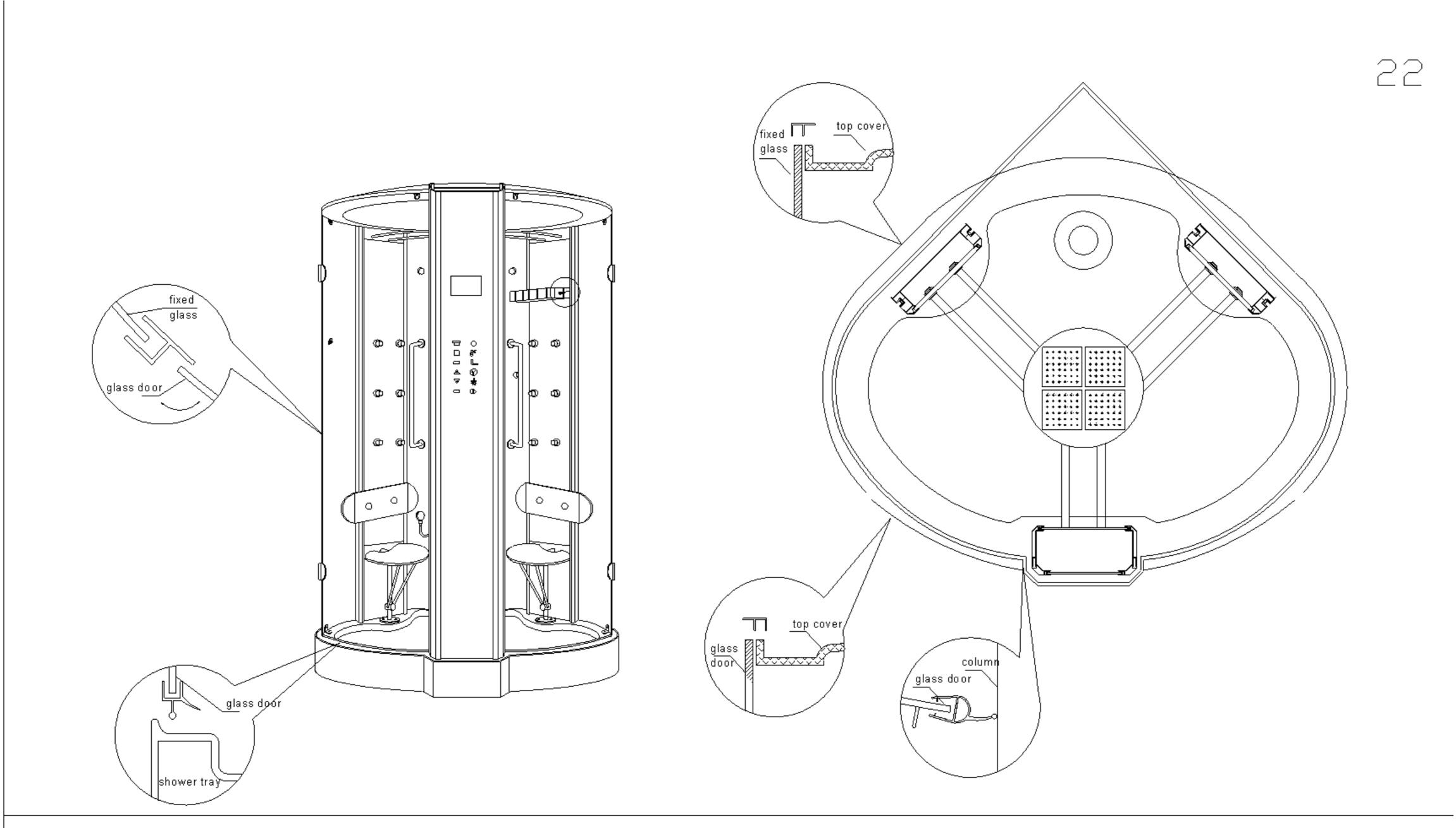
22. Install plastic seal: please install plastic seal as per picture shows to avoid water leakage and steam leakage.
