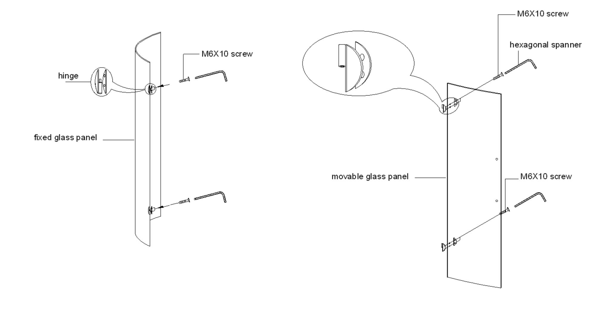
7. Install hinge for fixed glass panel and movable glass panel.
