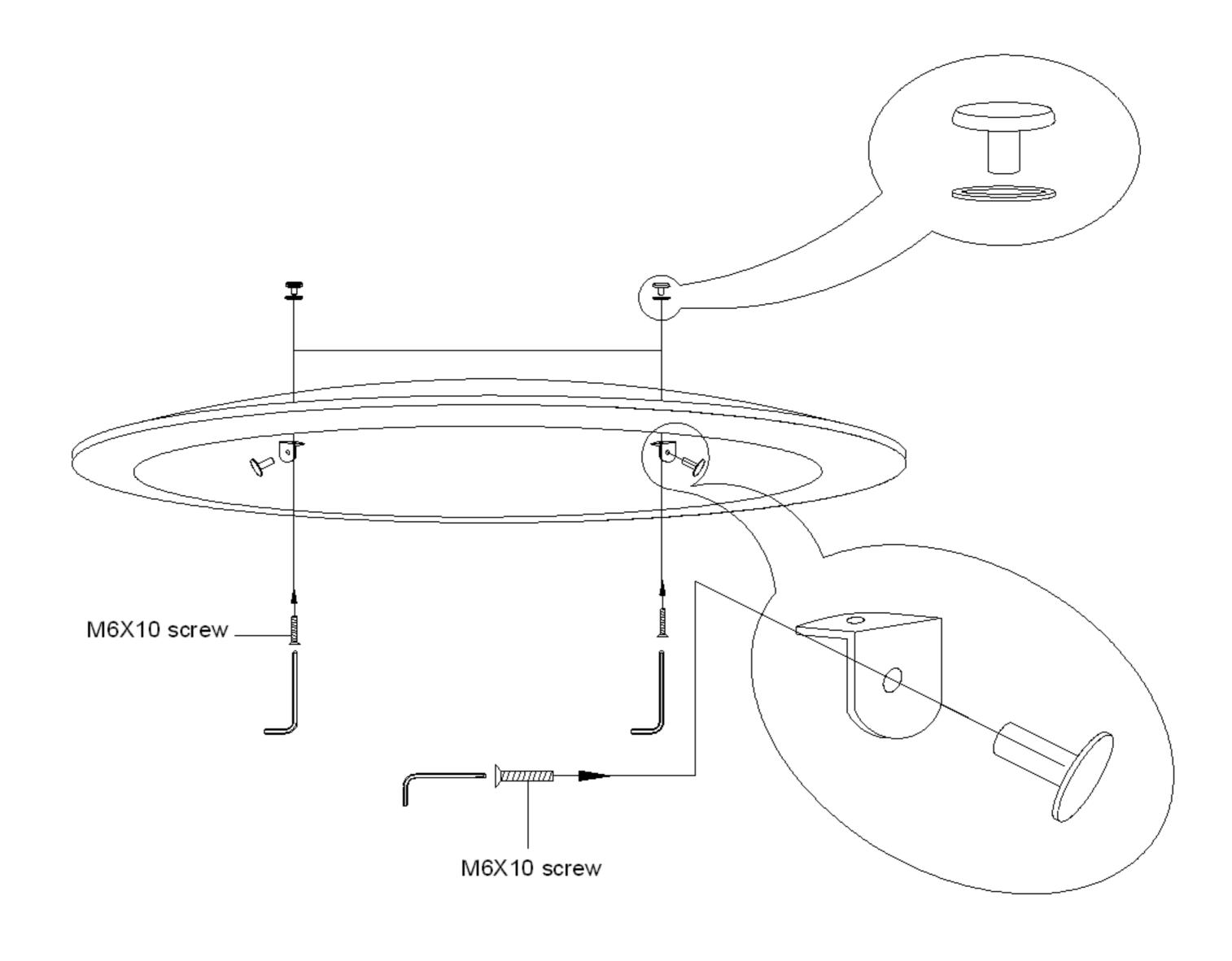
16. Install magnetic cylinder on top cover.
