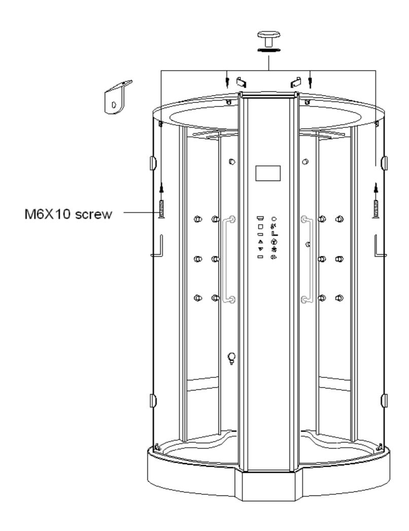
18.Get fixed glass panel and top cover connected. Get decorative aluminum profile wedged into the column.
