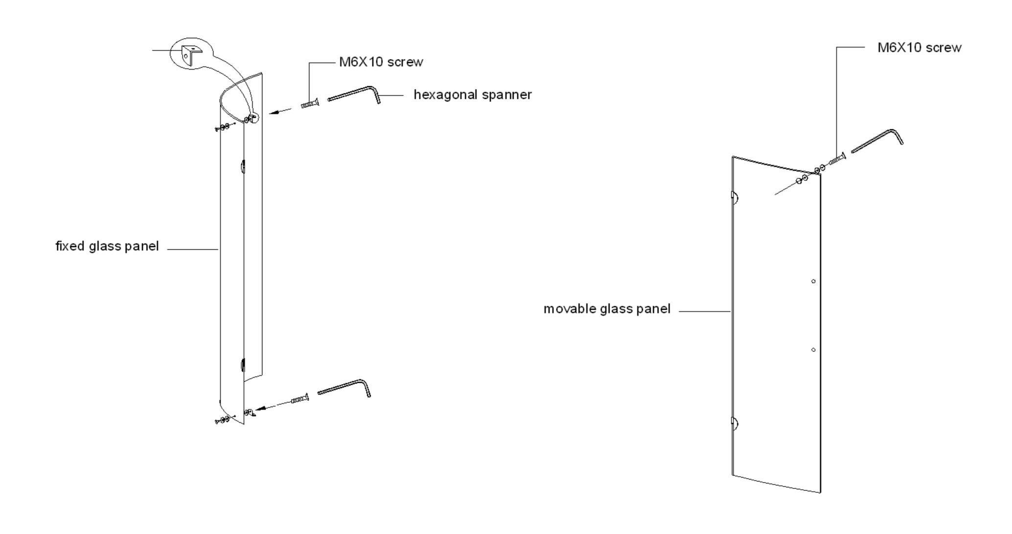
8. Install glass clip for fixed glass panel and magnetic cylinder for movable glass panel.
