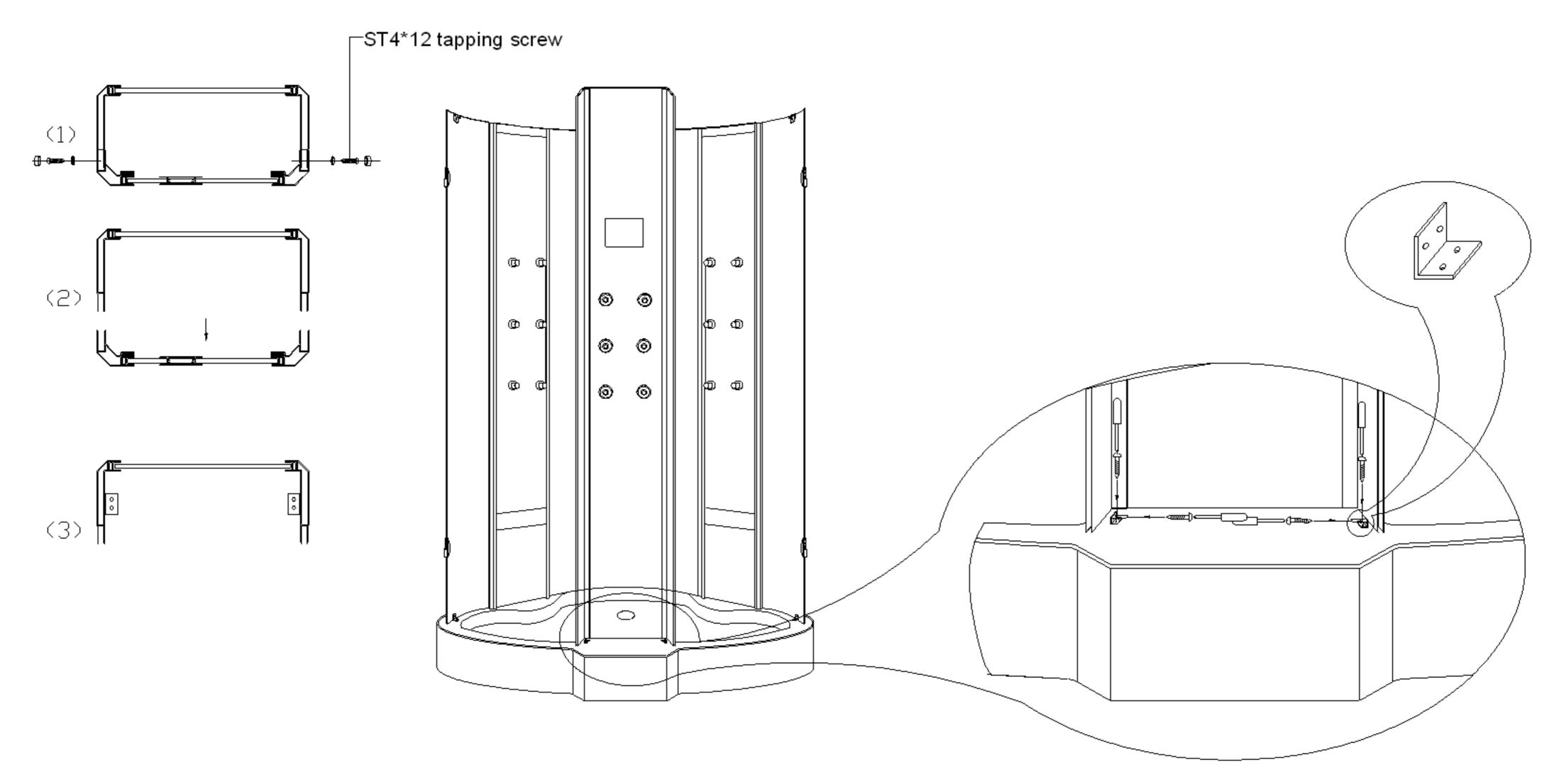
11. Install inside part for front column. Get water supply and power supply connected according to number.
