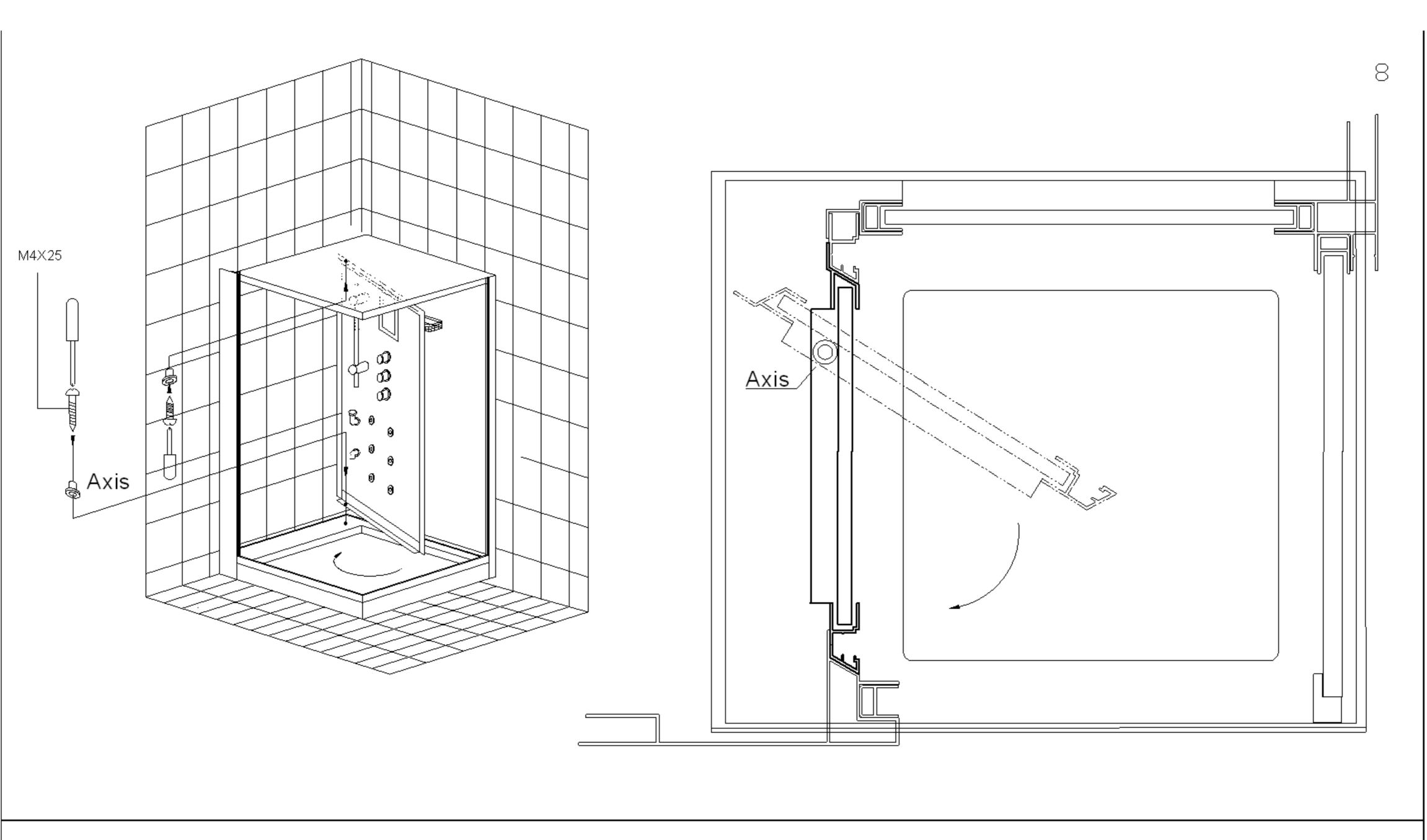
8. Install the back panel??Get the back panel connected to the shower tray with screw and axis.
