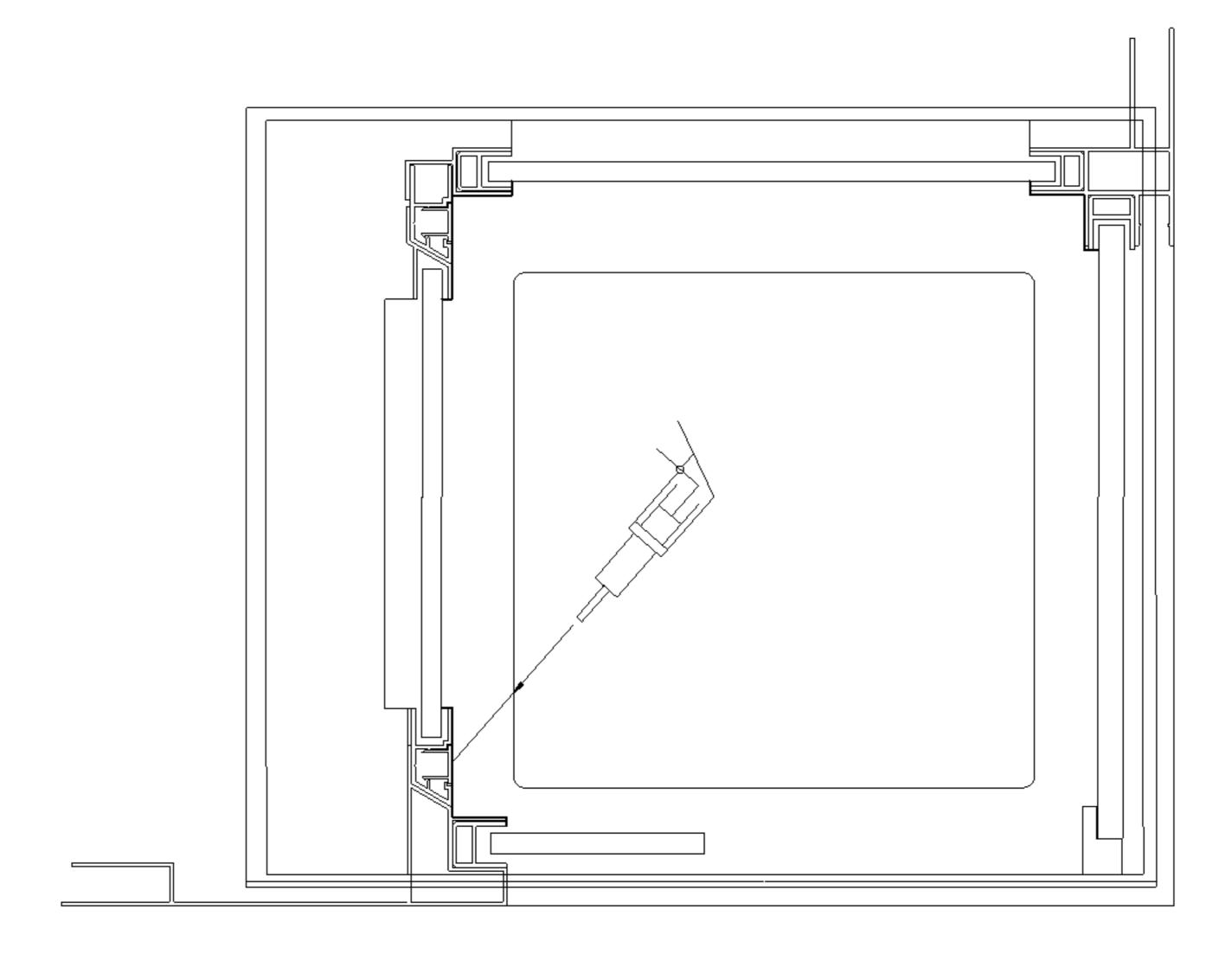
15. Apply silicone. No using within 24 hours
