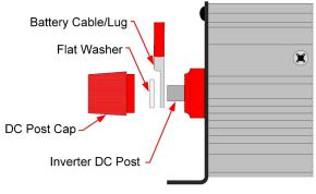
**IMPORTANT:** When fully tightened, the Cable Lug should not be able to rotate around the Inverter connection post. Check and tighten the end caps periodically as they can become loose from vibrations or thermal cycling.
