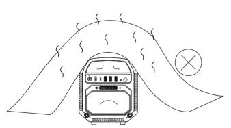
2. The Generator does not have an IP waterproof rating. Do not use in rain or in any other situations can get wet.
