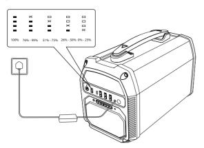
2.When you want to check the remaining power level under standby or while working, short press the main power button to check as below:
