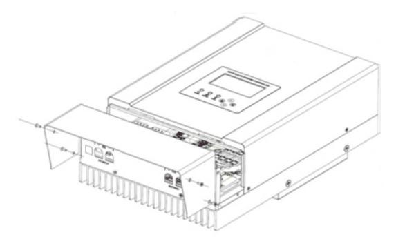
Use a #4 Phillips screw driver to remove the four screws that secure the wiring box cover as show in figure below.
