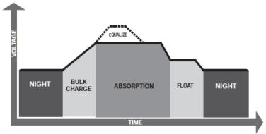
Figure 4-2. MPPT controller Charging Algorithm
