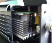
12. Replace the screws removed in Steps 1 & 2.
