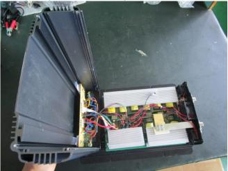
8. Using nipper pliers or a similar tool, gently pull out the fuse(s) to be replaced.
