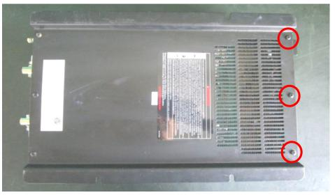
2. Remove all four screws on the DC end panel as shown below.
