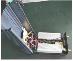
6. With a screwdriver remove the conductive "L-brace" as shown below. Note: Take care to not lose any of the screws being removed.
