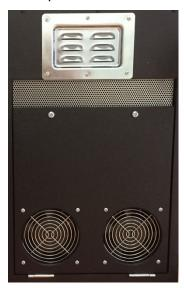
This is a photo of the area of the back panel where the cooling door is. The silver louvred and perforated exhaust plates are visible near the top and the two door securing machine screws are clearly visible just below the perforated exhaust plate.
