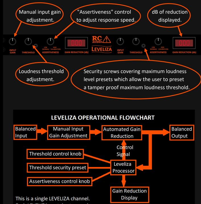
Each LEVELIZA contains two such identical and independant channels.
