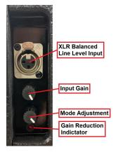
Input is via line level balanced XLR connector.
