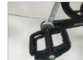
12. Take out the pedal with the letters "R" and "L", align it with the crank hole and lock it with a wrench
