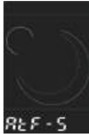
Automatic shutdown time settings interface
