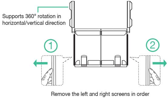
Note: To remove or store the screen, you need to erect the support pole and bracket to 90 degrees.
