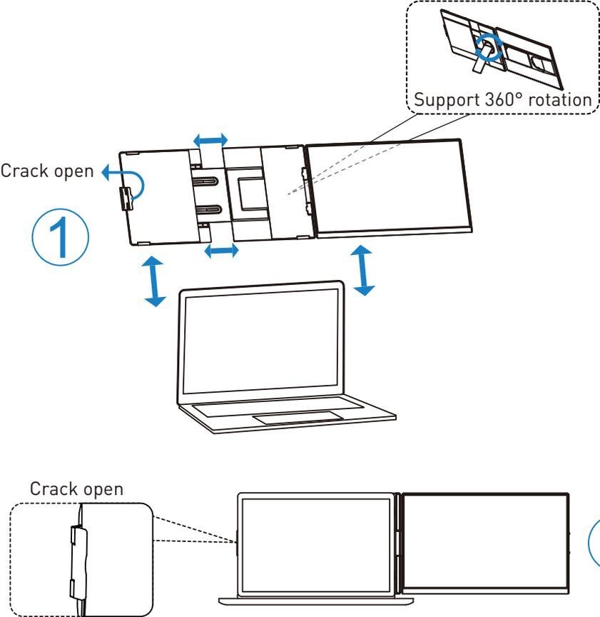
\*Note: Open the stand, adjust it to the appropriate supporting angle, place it behind the computer screen, and complete the installation of the dual-screen support.
