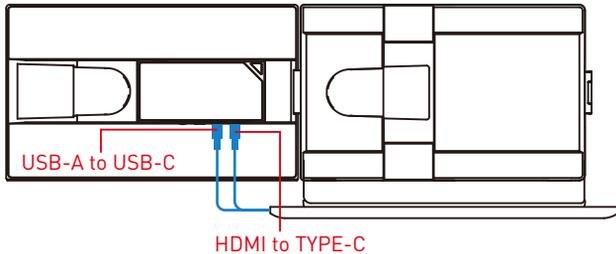
**Note:** The HDMI to TYPE-C cable must be connected to the third port of the screen extender for video, and the USB-A or USB-C to USB-C cable must be connected to the first or second port for power supply.
