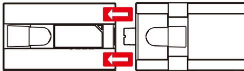
Note: Hold both red arrow positions with both hands and pull the screen outwards to remove the single screen for use.
