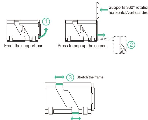
Note: The maximum stretching length of the bracket is 408mm
