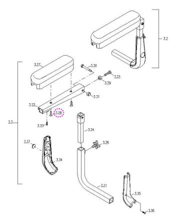
Note: The arm tube protective shrouds (3.34 and 3.35) are option parts for powerchair.
