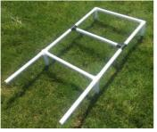
Repeat this process until all 9 rungs are built. Every other rung will have two short poles (A) extending down for stability. When the final rung is complete, use the white three-way connectors (E), to attach the final rung (C) with the two short poles (A).
