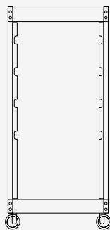
Trolley with slots in polished AISI 430 steel - dimensions: L327xW346xH901 equipped with Standard d.60 castors black/chromium plated without brake (shelves not included)
