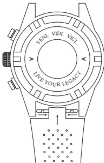
Pinch the two springbars together into the center of the strap & lift up to remove the strap from the case.
