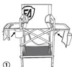
Lift up the side table and ensure supporting brackets are locked.
