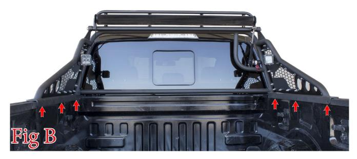
3. Line the mounting holes on the chase rack up with the newly drilled mounting holes on the bed rail. Then, use the supplied 1/2" Bolts (x6), 1/2" Washers (x12), Backing Plates (x6), and 1/2" Lock Nuts (x8). Mount the hardware exactly as shown in (Fig C). Once all bolts are loosely installed, torque the mounting bolts to 70 foot pounds.
