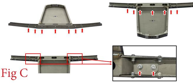
4. Locate the tire carrier arms. Secure the arms in place by loosely installing the supplied 3/8" Bolts (x6), 3/8" Washers (x6), and 3/8" Lock Nuts (x6). Make sure to mount the supplied plate between these arms. Once the arms are installed, go back and tighten all mounting bolts to 30 foot pounds. (Fig D)
