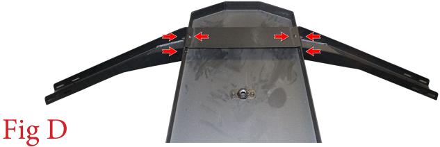
5. Find one of the tire carrier mounting pieces. Set it in place, then secure it loosely by installing the supplied 3/8" Bolts (x10), 3/8" Washers (x10), and 3/8" Lock Nuts (x10). (Fig E) We do not recommend installing the second mounting piece until the tire carrier portion is being installed on the truck.
