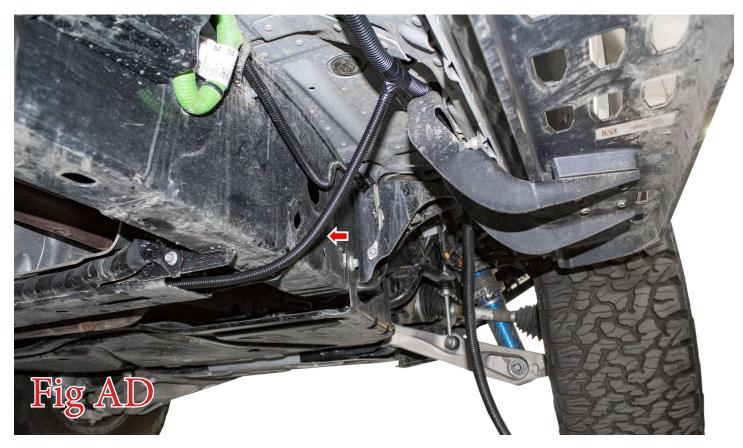
35. Using the supplied splice connector, connect the orange wire from the supplied harness to a wire on your vehicle that gets power when the brakes are applied. (Fig AE) shows how the splice connector works.
