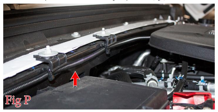
20. Remove this plug from the firewall. Then, drill a hole in it big enough to pass the wire harness through and reinstall it. (Fig Q)
