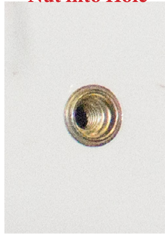
Push Rivet Nut into Hole
