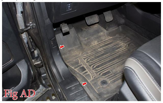
35. Lift the edge of the carpet and find the body plug that runs close to the door sill. Remove this body plug, cut a slit in it with a utility knife, then reinstall the plug. (Fig AE)
