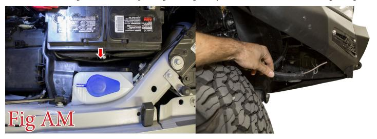
42. Find the wires for the side marker light. Split the conduit to expose the wires. (Fig AN)
