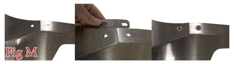
14. Go back and tighten all roof rack assembly to 30 foot pounds.
