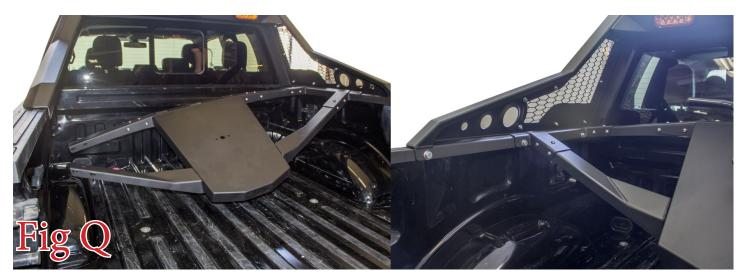
19. Set the roof rack section in place. Then, use the supplied 3/8" Bolts (x16), 3/8" Washers (x16), and 3/8" Lock Nuts (x16) to loosely secure it. The bolt holes can be accessed through the toolbox openings (the picture does not show all of the mounting bolts). Once all mounting bolts have been installed, torque them to 30 foot pounds.
