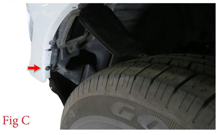
4. Remove the plastic clip holding the access panel down on the inner fender well. Then open the access panel. Do this on both sides of the vehicle. (Fig D)
