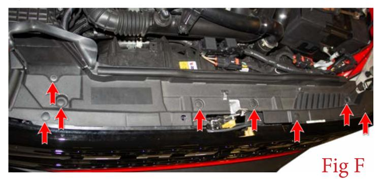
7. After the clips have been pulled out take out the shroud.
