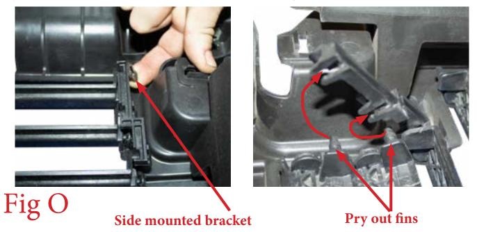
17. After the bracket has been taken off you will be able to take out the fins. We recommend using a flat head to pry out the fins on one side which will release the other side. You only need to take out the top 2 fins which the bracket held in place. After that you need to cut out the section shown in. (Fig P).
