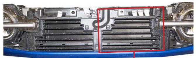
After the inner grille has been pulled out of Bronco,"-Fig L" shows how to take out the fins
