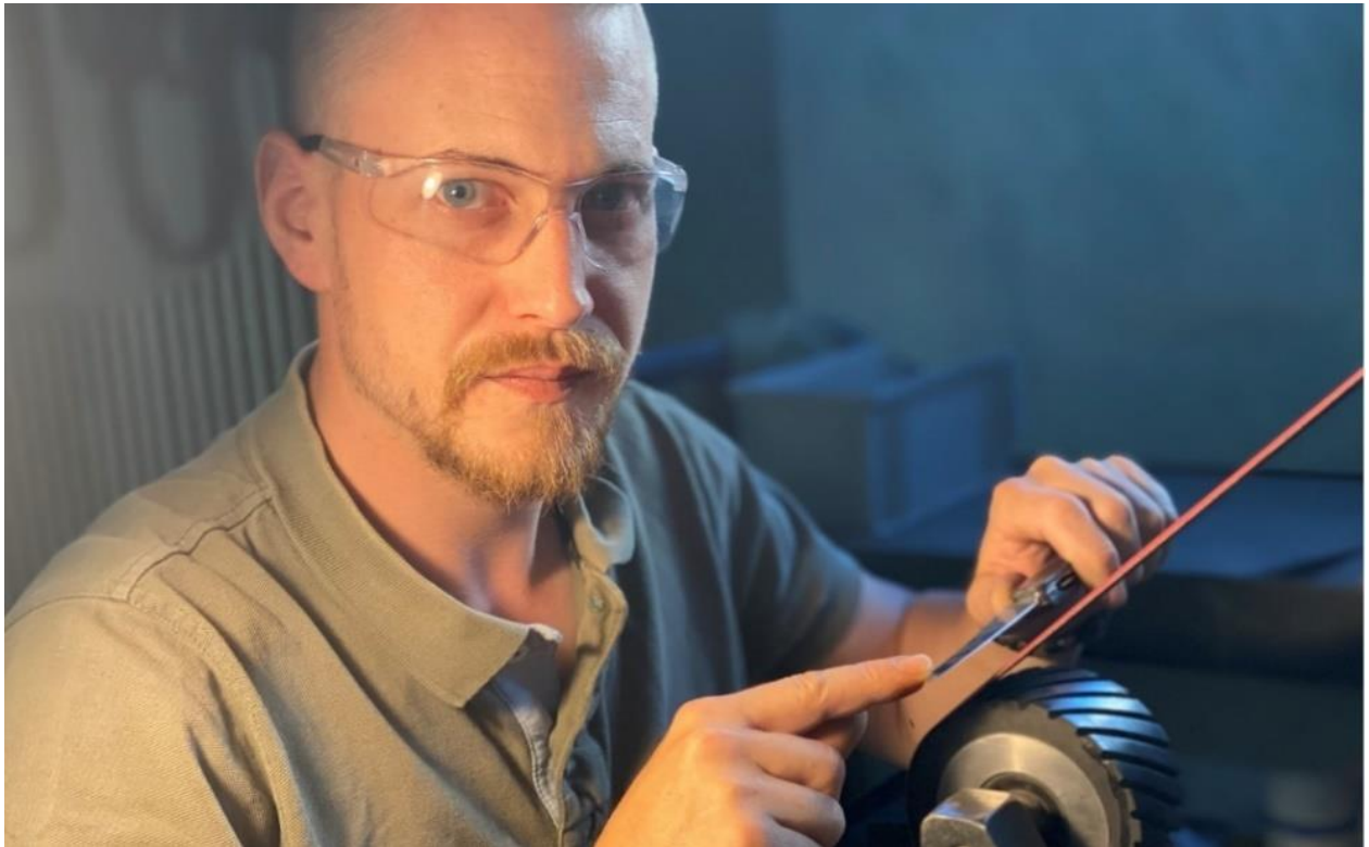
Cutler Timo Müller sharpening - one among more than 40 steps in knife production that are conducted by hand
