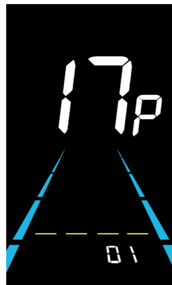
Figure 6-17 Controller cruise control setting interface
