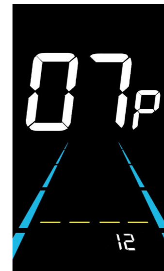
Figure 6-7 Number of speed sensor magnets setting interface
