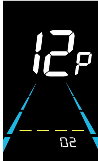
Figure 6-12 Pedal assist Start-up intensity setting interface
