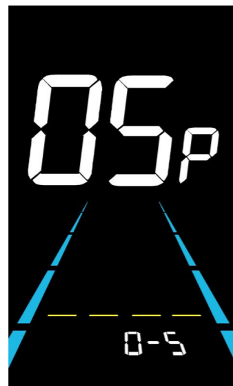
Figure 6-5 PAS level setting interface
