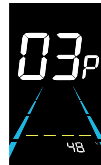
Figure 6-3 Rated voltage setting interface
