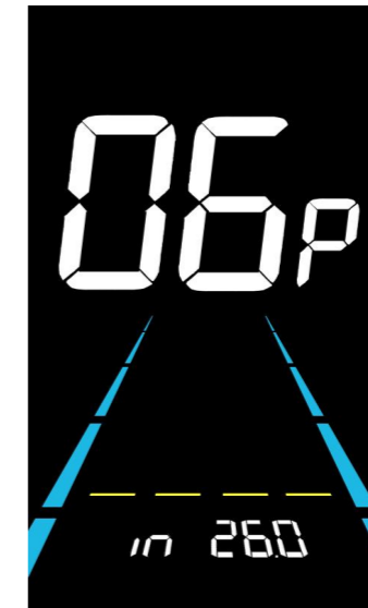
Figure 6-6 Wheel diameter setting interface
