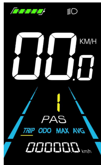
Figure 5-3 Backlight display interface
