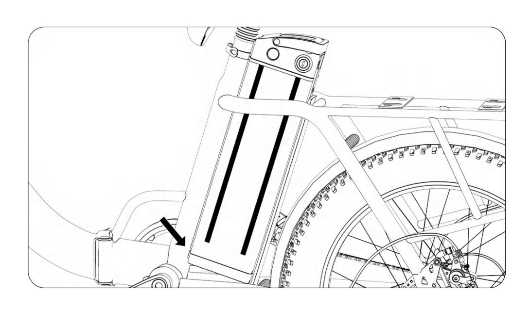
2. Insert the battery to the bottom, make it fully contact with the discharge plug.
