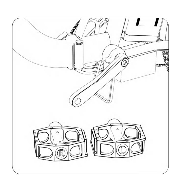
6. When installing the foot pedal, pay attention to distinguishing between "R" and "L".
