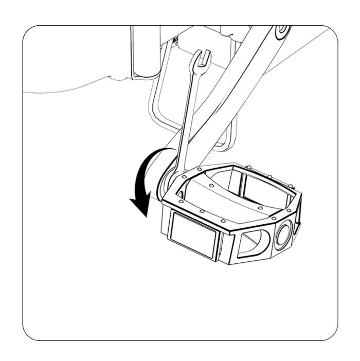
7. Use a wrench to tighten the pedal.
