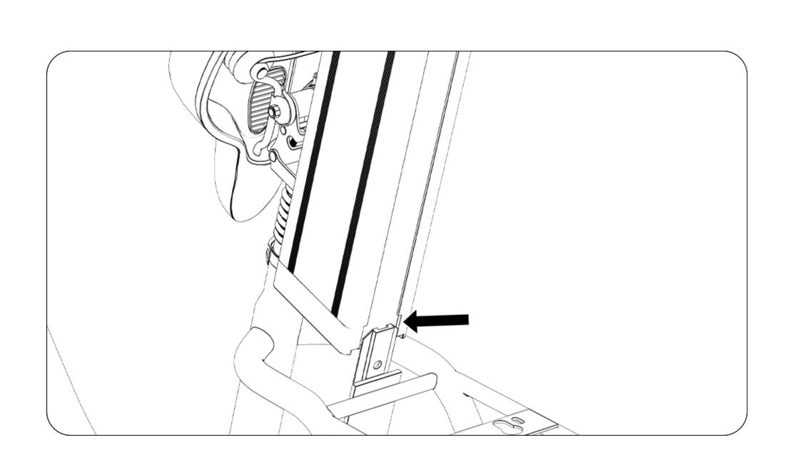
1. Align the groove on the back of the battery with the battery track.
