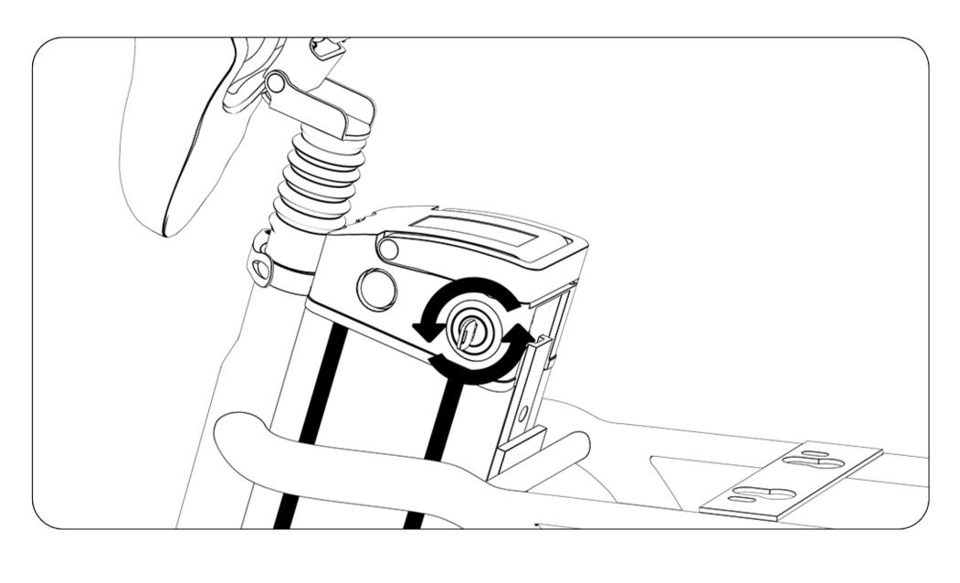
3. Turn the key to unlock the battery.
