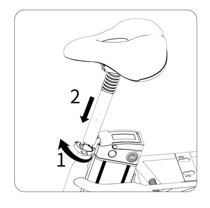
8. Open the telescopic adjustment latch and insert the seat in the direction of the arrow.
