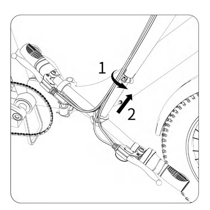
3. Open the folding tube telescopic adjustment latch, insert the telescopic tube in the direction of the arrow.
