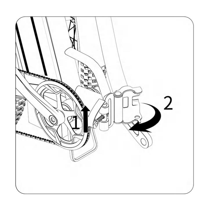
1. Push the folding handle upward and assemble the folding frame according to the arrows.
