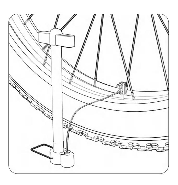
9. Inflate the front wheel slowly to prevent the tire from bulging out on both sides.
