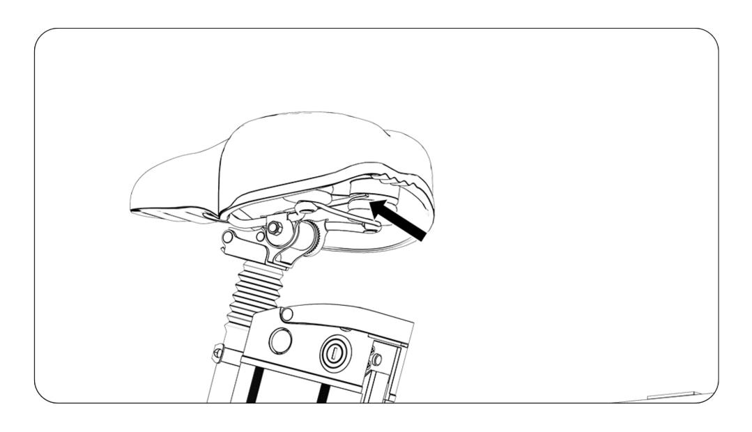
1. Pull up the handle at the bottom of the saddle.
