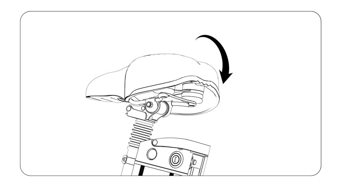
4. Put the seat down and hear the buckle sound, which means the seat is fixed.
