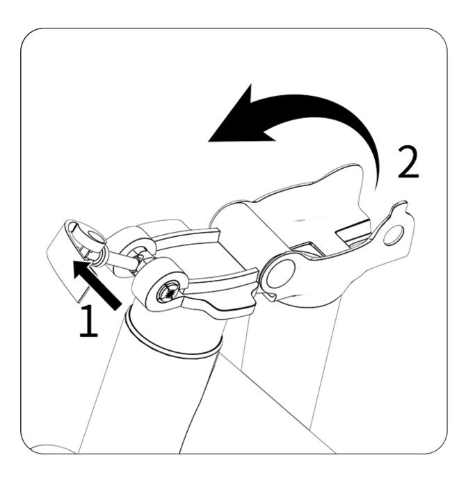
4. Push the folding handle according to the arrows, then fold the front frame of the bike according to the arrows.
