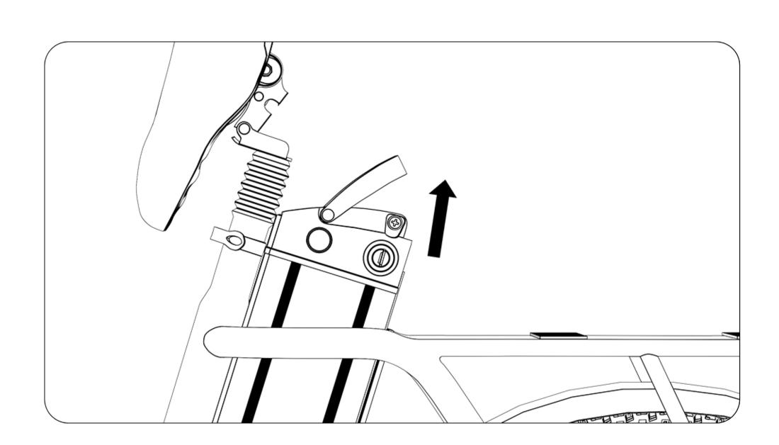
4. Pick up the battery handle and take out the battery.
