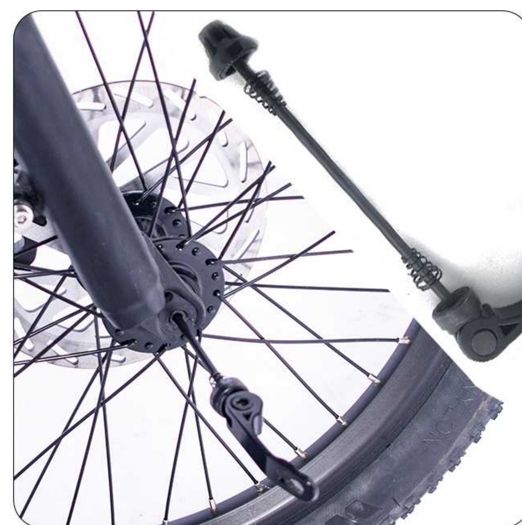
9. Install the front wheel quick release shaft as shown in the picture, with two conical springs, one on each side, with the smaller direction facing inwards. Finally, tighten the quick release shaft.
