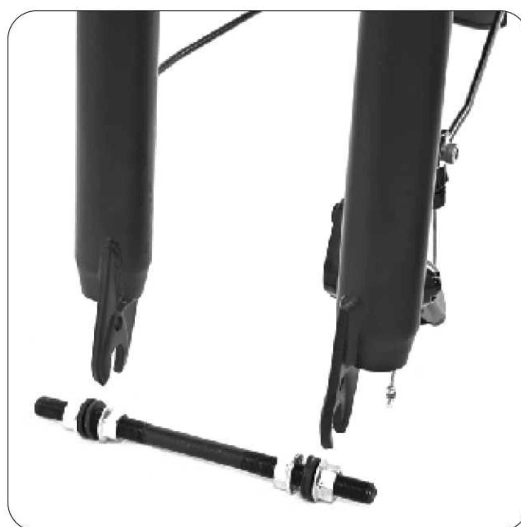
5. Remove the front wheel clip, then remove the front fork protection rod and brake protection pad.
