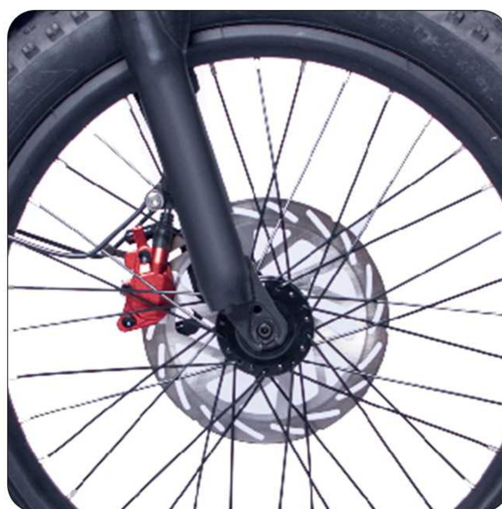
8. Install the front wheel, paying attention to the holes in the wheel and front fork, as well as the clearance for the front brake and brake pads.
