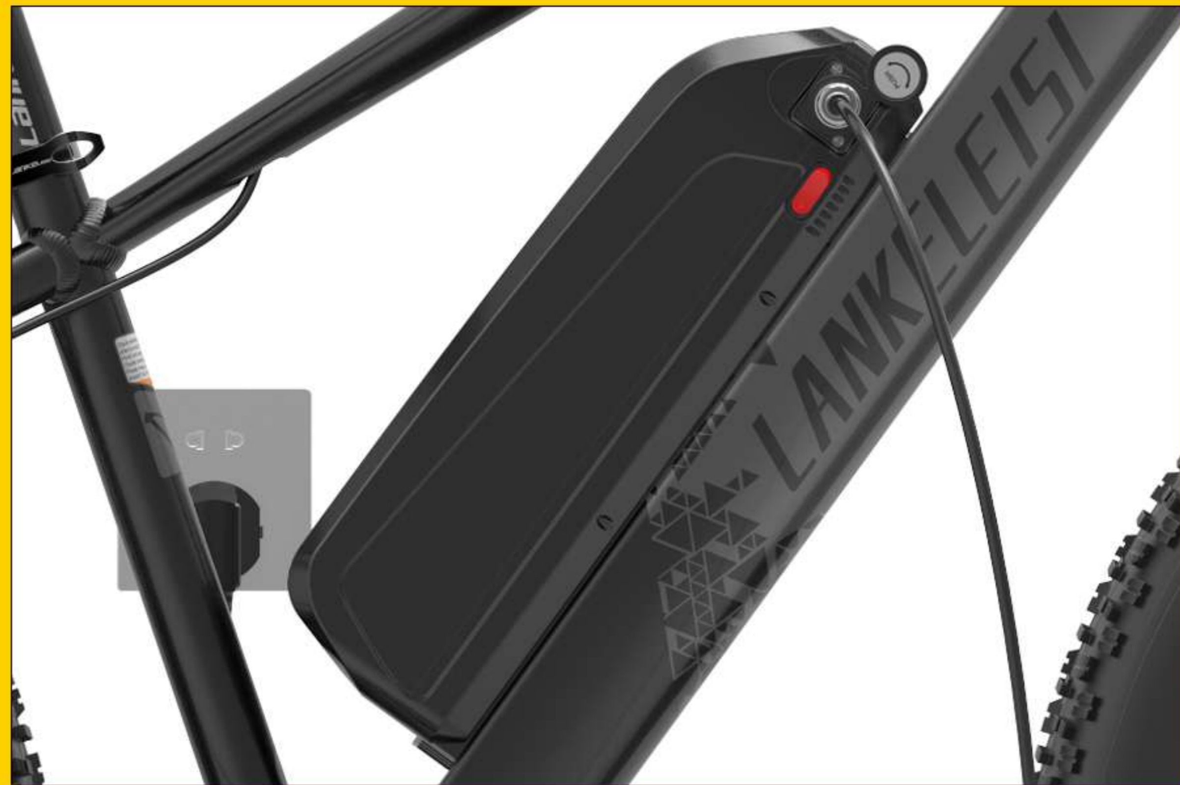
A. Recharge the battery on E-Bike directly
