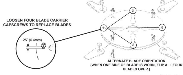
4. Replace, flip or sharpen blade and then loosely bolt blade into position on the carrier. (Install capscrews from the bottom up, with the lock nut towards the access opening.)
