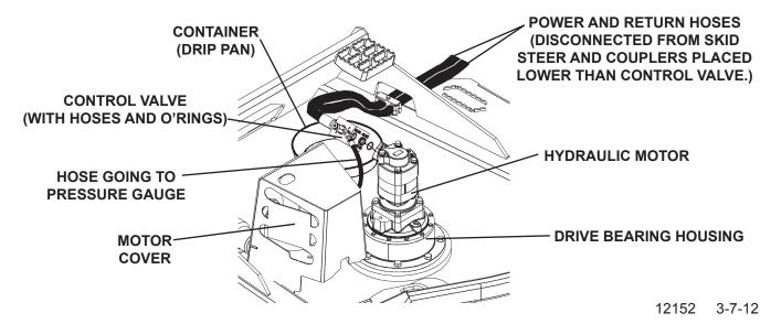
3. Remove the capscrews holding the motor to the drive bearing housing, and remove the motor. Check motor seal for damage and replace if required.
