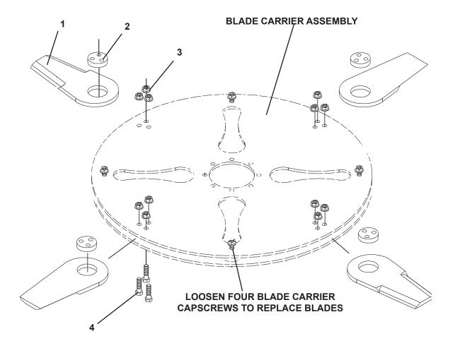
ALTERNATE BLADE ORIENTATION (WHEN ONE SIDE OF BLADE IS WORN, FLIP ALL FOUR BLADES OVER.)
