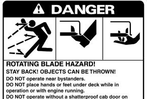
DO NOT operate without a shatterproof cab door on loader. Stop engine before leaving loader or servicing.
