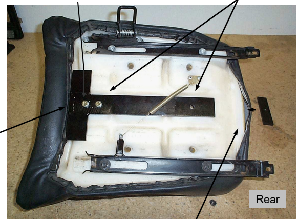
Remove staples to slide bar inside seat, to line up on hole. Use a small pry bar or large screw driver, to unglue foam from seat base. Staple cover back in place after bars are installed.
