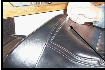
Step 3: Measure from front of seat back 1 1/2". Feel for and measure foam, not loose seat cover. Mark and center side to side. Will be centered between the real thread on band between front and rear seat on Cavalcade (see Step 3 below).
