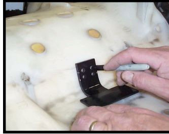
Step 1: Lay Bottom T-Bar in place, and mark holes onto seat base.
