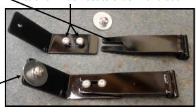
Step 2: Loosen the 2 bolts on the Seat Tray, with 13mm socket, back 2 full turns, or so, but not all the way out.
