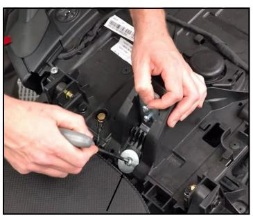
Step 5: Line up Hole in Mounting Bracket with Hole on bike. Insert Bolt with Lock Washer and Fender Washer, through hole into threaded hole in Mounting Bracket and tighten snuggly, but do not over tighten. Tighten Bolts in Step 2.
