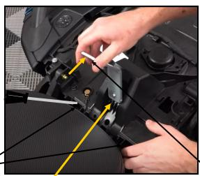
Step 4: Insert Utopia Mounting Bracket into receiver slot, as far as you can, on top of the 1" Square Bar under Seat Tray. With some force push back, or hit top of Mounting Bracket popping it in place on top of the 1" Square
