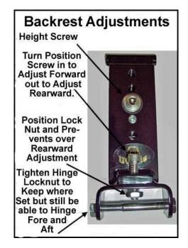
A driver's backrest that becomes part of your seat. No bars in the way of the driver's hips and legs or passenger's legs. Folds forward to ease passenger getting on or off and adds to safety by getting out of the way in sudden stops. Has up and down height adjustments, as well as driver seating position, back and forth, to help driver sit upright to avoid slouching, a big factor in driver fatigue. Included is our Quickout, that allows you to pull up on Backrest to remove.
