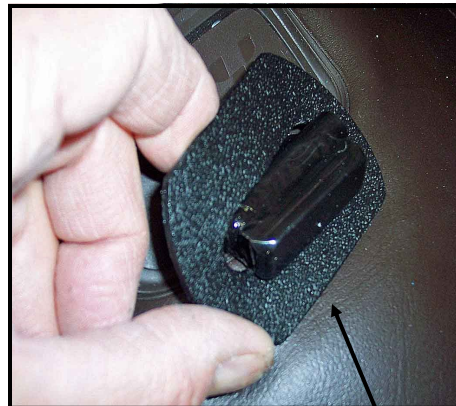
Step 17: Peel off paper from adhesive tape, on our boot. Work our plastic boot over tube on mounting bracket, with adhesive toward rear. May need to struggle some, but will go on. If boot sticks as you install, just release until you have in place.
