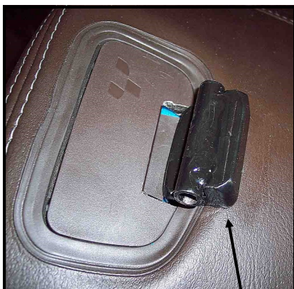
Step 16: Plastic hole cover now in place. With rubbing alcohol clean seat cover behind bar, for next step.
