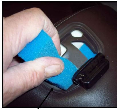
Step 12: Stuff entire foam pieces furnished into the O.E.M holes. Do not worry about stuffing all the way to bottom, just make level with top. This fills void, firming up seat.
