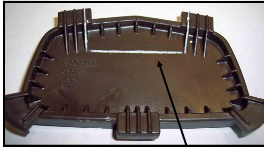
Step 2: On back side of cover mark lines as shown. Cut out will look bigger than necessary, but bigger for a reason. It allows for movement of cover when you compress foam in front of cover. If smaller it will buckle against mounting bracket.
