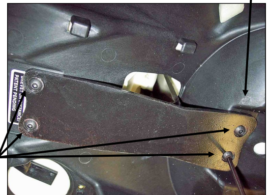
Step 10: Insert screws furnished through mounting bracket into threaded holes in seat base. Tighten screws with 5/32 Allen wrench.
