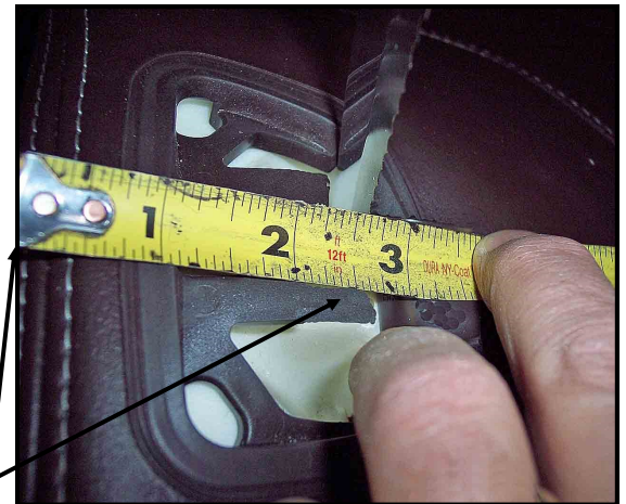
Step 8: With long serrated knife cut slit in foam connecting holes already in foam all the way through to bottom of seat through hole in seat base, approx. 2 3/4" from front edge.
