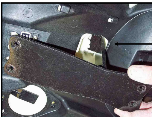
Step 9: Slide mounting bracket through hole in seat base, into foam you slit, up through top of seat.
