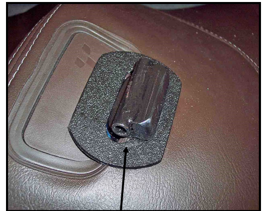
Step 18: Make sure boot is all the way forward, tight up against back of mounting bracket. There is no adhesive on front of boot, to allow hole cover to move back and forth with foam compression when you push back into driver's seat.
