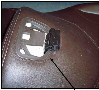
Step 11: Close seat. Bar should now look like this, coming out of seat.
