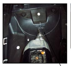
Step 2: Drill 9/32" Holes (slightly bigger than 1/4") in Seat Base that You just Marked in step 1
