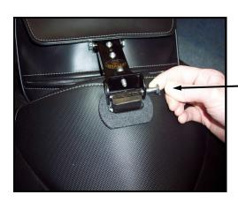
Step 8: Finally, install bar attached to pad to tube now sticking out of seat. Slide in 2 1/4" bolt furnished and tighten nut. Make tight enough that backrest will stay in place, but will still hinge back and forth.
