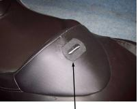
Step 4: Peel backing off Boot and Stick Boot in place Centered over Mark You just made on your seat in step 3.
