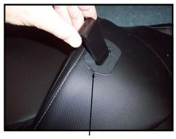
Step 6: With Tube toward front of seat, Slide Inside Bar into Slit, from Top of Seat, through Boot into Foam until Bar hits bottom and Tube rests on Boot.
