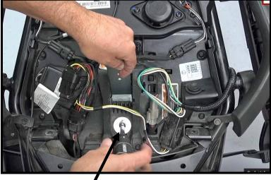
Step 4: Insert bolt with lock washer and fender washer, through hole into threaded hole in Mounting bracket and tighten snuggly, but do not over tighten.
