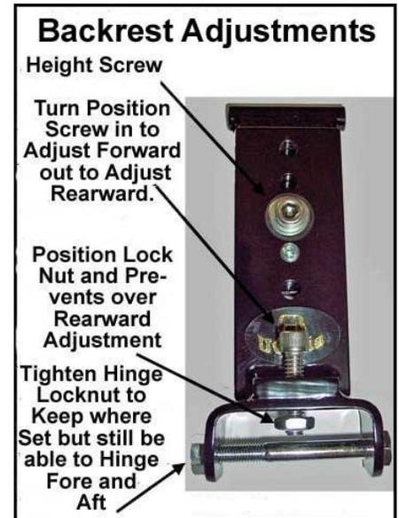
A driver's backrest that becomes part of your seat. No bars in the way of the driver's hips and legs or passenger's legs. Folds forward to ease passenger getting on or off and adds to safety by getting out of the way in sudden stops. Includes up and down height adjustments, as well as driver seating position, back and forth, to help driver sit upright to avoid slouching, a big factor in driver fatigue.
