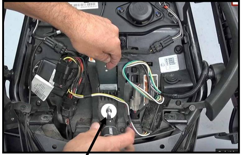
**Step 4:** Insert bolt with lock washer and fender washer, through hole into threaded hole in Mounting bracket and tighten snugly, but do not over tighten.
