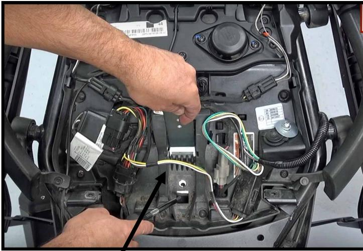
**Step 3:** Slide mounting bracket into receiver slot under seat. Line up hole in mounting bracket with hole in receiver.
