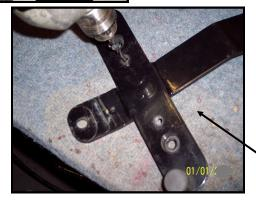
Step 4: Drill 11/32" hole, or a bit slightly bigger than the 5/16" bolts furnished. Can also use drill press if available.
