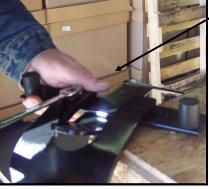
Step 7: Finally, with seat installed on your bike, install bar attached to pad to tube on Utopia Bracket you just installed on your seat. Slide in 2 1/4" bolt furnished and tighten nut. Make tight enough that backrest will stay in place, but will still hinge back and forth. Adjust Utopia Driver Backrest for Comfort and take a ride!!!!
