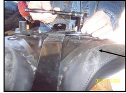
Step 3: Remove bracket attached to bottom of seat, by removing 2 nuts on rear and 1 bolt on front.
