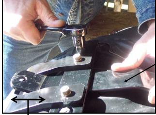
\*NOTE: Shown in normal install position, but can move bar forward or backward to move closer or away from back of seat, before marking to drill in step 2. Rarely would want to move backward, but for a two up seat moving forward will help with clearance between front and rear seats.
