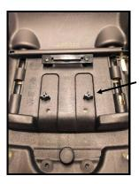
Step 1: Place on your workbench buttom up. Remove the 2 Philips screws, holding the rear tool clip. You will re-install later in Step 6.
