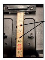
Step 2: Measure back 1 1/2" and 2 3/4" from front tool clip and mark centers. Drill through Seat Base, with 9/32 drill bit where you marked.
