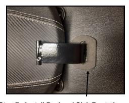
Step 7: Install Peel and Sick Boot, then slide Butt Pad into rear position.
