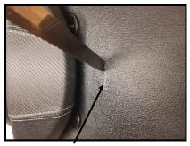
Step 4: Slide butt pad forward to assure you do not damage when you make slit in rear seat cover. With a serrated knife and cut through seat cover and foam all the way down to the seat base. Work knife tip side to side to make sure foam is clear of seat base. Do not cut wider than 1 1/2"
