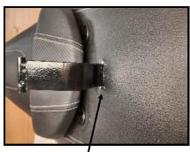
Step 5: Now slide mounting bracket into slit, all the way down to seat base, working it in between foam and seat base. Line up holes in Mounting Bracket with holes you drilled in Step 2, on bottom of seat.
