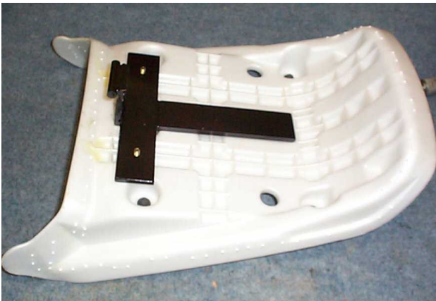
This is a photo showing the location of the supporting bracket in place on the plastic
