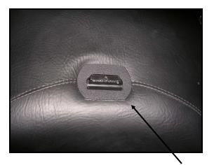
Step 4: Install the Peel and Stick Boot included with your new Backrest, over the Tube now above seat. This will protect your seat cover from Backrest hinge action. (will not use boot with the Quick Out Option)
