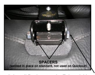
Step 5: Install Backrest to the Tube sticking out of Seat with the Bolt and Lock Nut Included.
