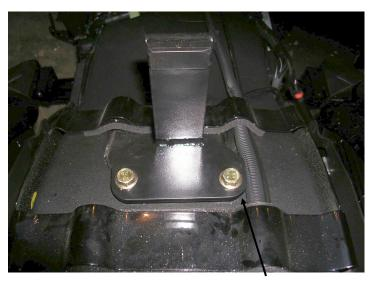
Step 2: Place Utopia Driver Backrest Bracket as shown, Install and Tighten the Bolts you removed from Passenger Strap Hardware, you just removed.
