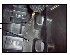
Step 4: Turn seat right side up. Trim holes in seat cover, that you just drilled, slightly bigger, cleaning any plastic seat base shavings from hole.
