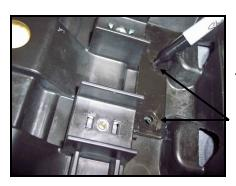
Step 2: With Stock Adjustable Pad now removed, lay furnished bottom bracket as shown and mark the holes onto seat base bottom.
