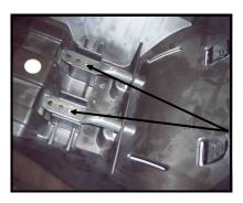
Step 1: Turn seat upside down. Find the small Phillips screws, shown here, for Stock Adjustable Pad Bracket. Remove screws, will reinstall later. Now Remove Stock Adjustable Pad.
