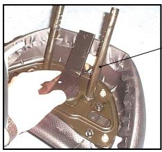
Step 11: From bottom of stock seat pad, push inside bar into the slit you made in step 4. Make sure the tube on inside bar is facing the front of stock pad and the extension is toward the rear. Push helping the tube extend through slit you made in cover on top.
