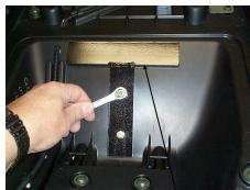
Step 14: Turn seat over again. Line up Anti-Flex Bar, with holes you drilled, with drop in "T", down toward the seat base. Insert bolts with lock washers and tighten. (Will help to use small Phillips Screw driver in one hole while placing bolt in other).
