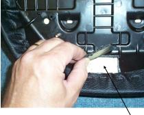
Step 4: Remove and discard plastic piece you just cut out. May need to pry up with straight edge screw driver first.
