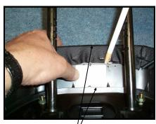
Step 2: Center template 2 3/4" from edge of pad to bottom of template. Mark around template with pencil or pen.
