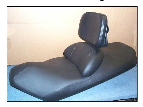
A driver's backrest that becomes part of your seat. No bars in the way of the driver's hips and legs or passenger's legs. Folds forward to ease passenger getting on or off and adds to safety by getting out of the way in sudden stops. Includes up and down height adjustments, as well as driver seating position, back and forth, to help driver sit upright to avoid slouching, a big factor in driver fatigue.
