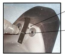
Step 7: Push small part of inside bar into slot as far as possible, being sure bar is centered from top to bottom..
