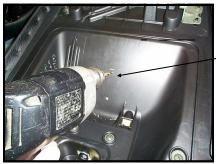
Step 9: Turn seat over and re-drill the holes you just drilled, with 9/32" bit.
