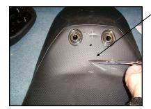
Step 10: Turn seat right side up again. With scissors trim cover at both holes, about 1/2" in diameter. This will assure vinyl is out of the way when you insert the bolts later.
