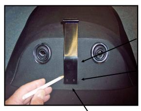
Step 5: Using inside bar as template, rest small extension on back of bar on ridge of seat, centered on seat as shown. With pencil or marker mark around the bottom of bar onto seat cover.
