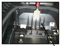
Step 9: With sharp wood chisel, remove about 1" of center ridge, just below the holes you just drilled, to allow anti-flex bar to rest in area.
