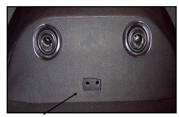
Step 6: Cut cover away from area you just marked. Place inside bar back on ridge, center, and mark the holes in bar onto seat base. Drill holes marked with 9/32" drill bit.
