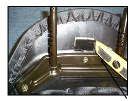
Step 3: With new blade in box knife, or cutter of choice, carefully cut out plastic in area you just drew. (Too deep will cut cover)
