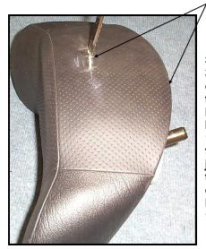
Step 4: Measure 3 3/4" from edge of pad and center a mark. With long serrated knife, cut slit 1 1/2" long aiming for the area you just cut the plastic out of. Be careful not to cut longer than 1 1/2".
