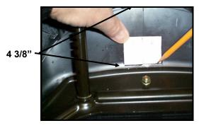
Step 2: Center template 4 3/8" from edge of pad to bottom of template. Mark around template with pencil or pen.
