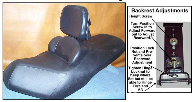
A driver's backrest that becomes part of your seat. No bars in the way of the driver's hips and legs or passenger's legs. Folds forward to ease passenger getting on or off and adds to safety by getting out of the way in sudden stops. Includes up and down height adjustments, as well as driver seating position, back and forth, to help driver sit upright to avoid slouching, a big factor in driver fatigue.
