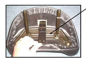
Step 7: From bottom of stock seat pad, push inside bar into the slit you made in step 4. Make sure the tube on inside bar is facing the front of stock pad and the small extension is toward the rear. Push helping the tube extend through slit you made in cover on top. Stop about 1" above cover for now.
