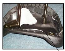
Step 1: With staple puller or straight edge screw driver, remove staples and vinyl backing on stock pad, that you just removed from seat and discard.
