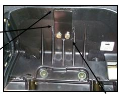
Step 9: With seat upside down, push down on seat forcing inside bar to slide in place. Line up holes, placing anti-flex bar in place, insert bolts supplied into holes and tighten into threaded holes in inside bar.
